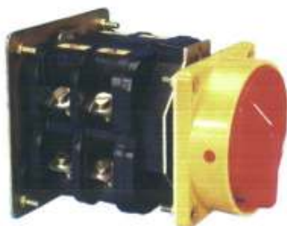
BASE MOUNTING THRO' 4 NOS. M6 SCREWS AT 100 CRS. FITTED WITH YELLOW RECESSED CUP & RED TOGGLE KNOB FOR PAD LOCKING
