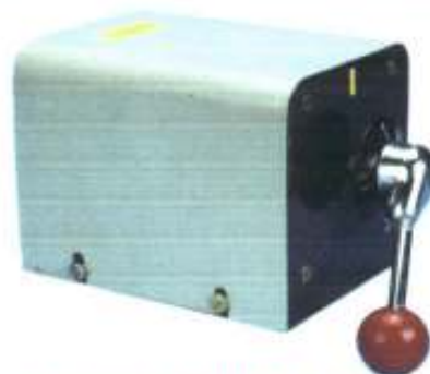
FITTED IN SHEET STEEL ENCLOSURE OPERATED THRO' SEIMENS TYPE INDEXABLE BALL HANDLE & ENGRAVED SKIRT MOUNTING THRO' 4 M6 SCREWS AT 122 x 82 CRS AT BOTTOM
